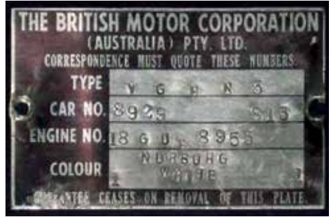
Pic 1 '8929' is the UK chassis number, whereas 'YGHN3 815' is the Australian identifier.
