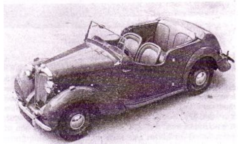
Comparatively few 'Y' type tourers (above) were built and those were all for export. The 'YB' saloon (below) proved much more popular. It had twin carburettors and externally could be distinguished by the smaller wheels, fatter tyres and deeper wing valances.
